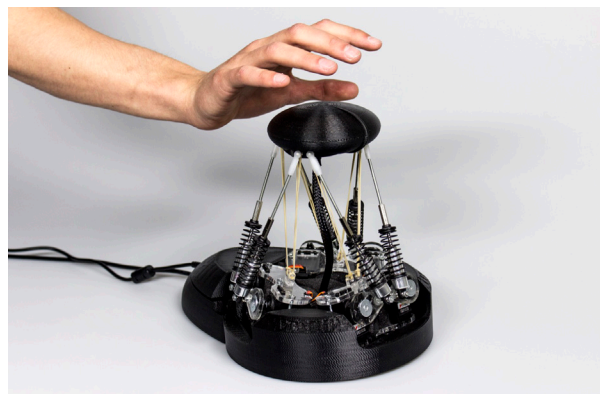
Figure 8. Stewart a haptic interface. In a project by Felix Ros (in Terken et al., 2016), a haptic interface named Stewart was developed allowing the user to sense and physically influence the behaviour and intentions of a fully automated vehicle. A form of haptic interaction was chosen since it was believed that it would be a non-obtrusive way to communicate the car's intention and also provide opportunities to indirectly influence the car's driving behavior. When driving, Stewart should enable people to do something else besides driving while providing a sense of control over the car's behavior.
