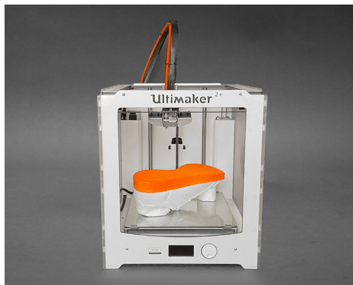
Figure 7. Shoe exploration #3 Replenishing AB plastic sole (in orange) with a 3D printer.
