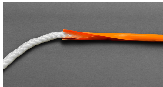
Figure 5. Rope exploration #1 AB plastic protective rope sleeve (in orange) around rope.
