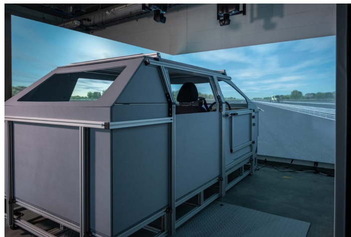
Figure 1. The vehicle buck and the simulator running SCANeR Studio.
