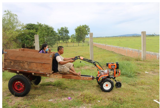
Figure 6. Project 2 Case 1 final product, cassava harvesting cart for people with mobility impairment. This reduces the amount of walking, bending, and carrying of heavy loads during cassava harvesting.
