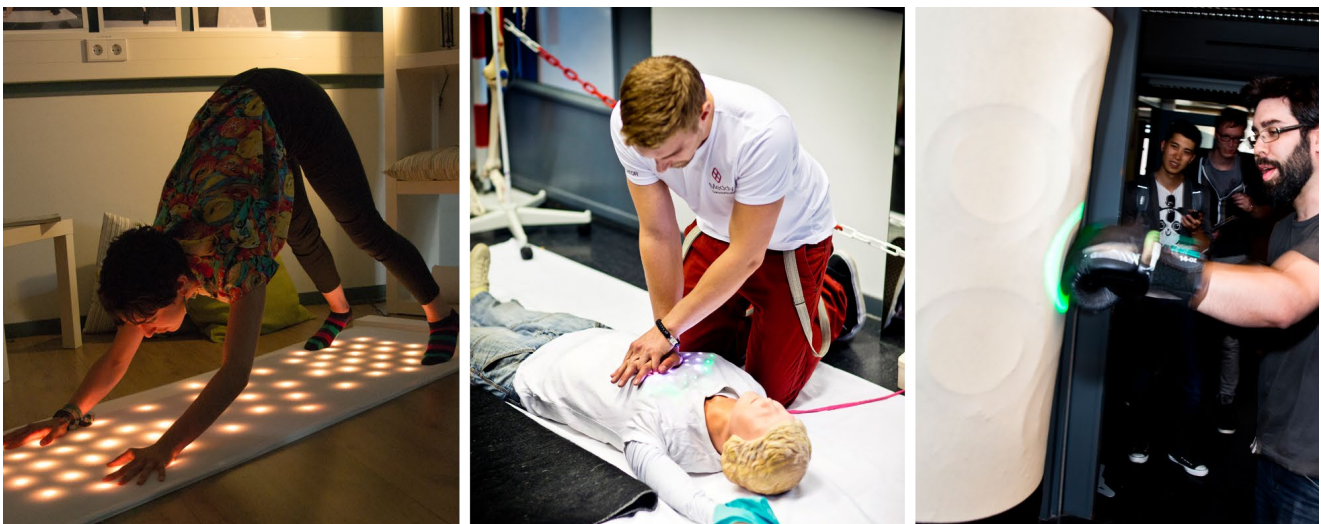
Figure 3. The integration of light and material elements in three final prototypes: Yoga mat (left), CPR trainer (middle), punching bag (right).
