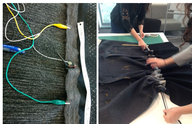
Figure 4. Left: Testing sensor conductivity. Right: Testing the tie/pulling mechanism and sensor activation.
