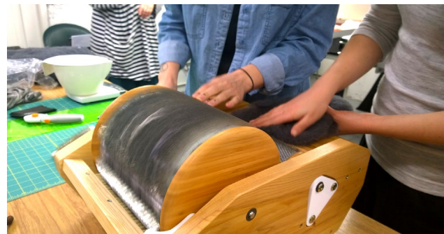
Figure 2. Carding wool and conductive fibers.
